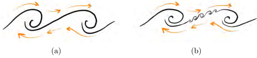
Figure 2: Schematic of the Kelvin-Helmholtz instability, with orange arrows indicating flow velocity. Panel (a) illustrates the primary instability, and panel (b) illustrates secondary shear instabilities on the braid of the primary instability.
