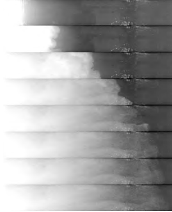
Figure 14: Time series showing, from top to bottom, the propagation of a turbidity current as seen from above ( m_g = 12.1 g, in the lock C_{\text{surf}} = 0.229 g/L while the rest of the tank was devoid of surfactant). The time lapse between two snapshots is \Delta t = 2.67 s and the horizontal length of each image is 97 cm.
