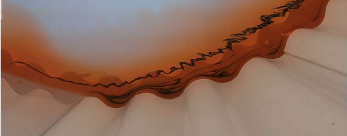
Figure 15: Photo taken from a GoPro camera mounted directly above the wavy wall near the source in an experiment with f = 2.5\text{s}^{-1} , g = 4.7\text{cm s}^{-2} , Q = 10\text{cm}^3\text{s}^{-1} , H = 14.9\text{cm} .
