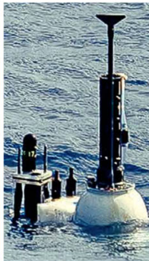
OSU chi-pod on a SOLO profiling float
