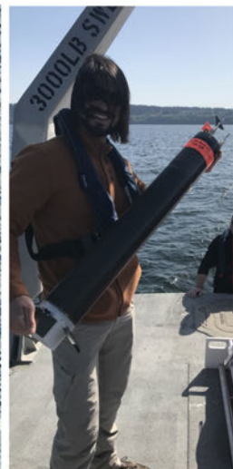
RSI "MicroRider" on an ALAMO (air-launched profiling float)
