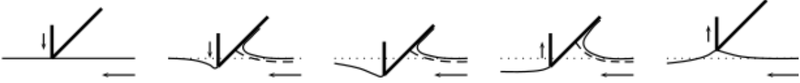
Figure 14: Snapshots of paddle and free surface over the course of a collision showing the evolution of the splash-up region ahead of the paddle.
