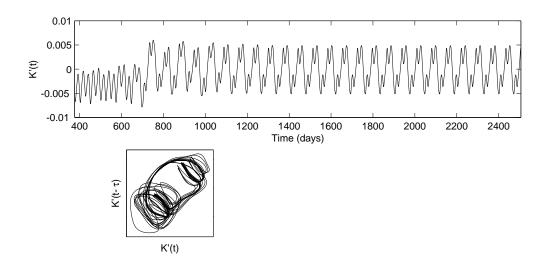
Figure 15: Time dependence of K' with  $Ro = 2.79 \times 10^{-2}$  for an integration started from branch 1 initial conditions, but which results in a final state on branch 2. Top: time series; bottom : delay-space trajectory for the time series.
