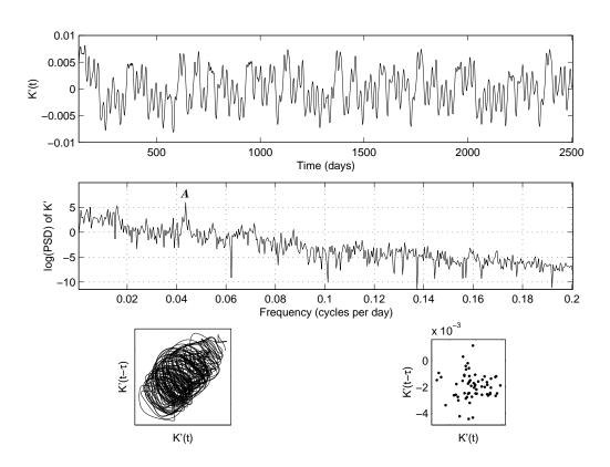
Figure 18: Time dependence of K' with  $Ro = 3.0 \times 10^{-2}$  for an integration started from branch 1 initial conditions. Top: time series; middle: power spectrum of time series (the zero frequency peak has been suppressed); bottom left: delay-space trajectory for the time series; bottom right: Poincaré section of the delay-space trajectory.
