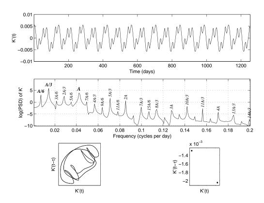
Figure 14: Time dependence of K' with  $Ro = 2.83 \times 10^{-2}$ , on branch 2. Top: time series; middle: power spectrum of time series (the zero frequency peak has been suppressed); bottom left: delay-space trajectory for the time series; bottom right: Poincaré section of the delay-space trajectory.
