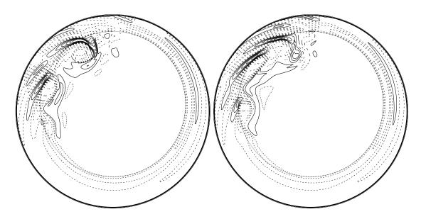
Figure 9: Contours of  $\zeta$  at two different times for  $Ro = 2.5 \times 10^{-2}$ . Left: at a local maximum of K; right: at the subsequent minimum of K. Contours of negative  $\zeta$  are dashed. Note how the strong anticyclone wraps a tongue of cyclonic vorticity around itself, which sheds a cyclonic eddy when the anticyclone dissipates. An animation of this sequence can be viewed at http://rses.anu.edu.au/gfd/link/AK/WHOIGFD.html
