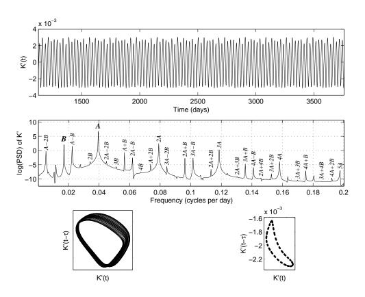
Figure 11: Time dependence of K' with  $Ro = 2.64 \times 10^{-2}$ . Top: time series; middle: power spectrum of time series (the zero frequency peak has been suppressed); bottom left: delay-space trajectory for the time series; bottom right: Poincaré section of the delay-space trajectory.
