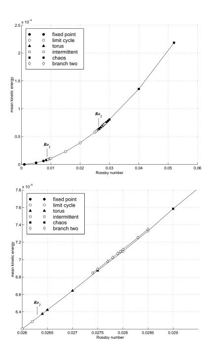
Figure 3: Time average  $\bar{K}$  of the basin-integrated kinetic energy as a function of Ro. a) the complete range of Ro investigated; b) a closeup of the transition from a limit cycle to chaos, showing the presence of two branches for a range of Ro.
