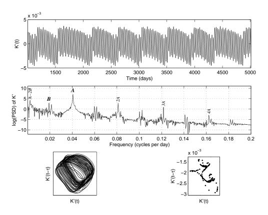
Figure 12: Time dependence of K' with  $Ro = 2.75 \times 10^{-2}$ . Top: time series; middle: power spectrum of time series (the zero frequency peak has been suppressed); bottom left: delay-space trajectory for the time series; bottom right: Poincaré section of the delay-space trajectory.
