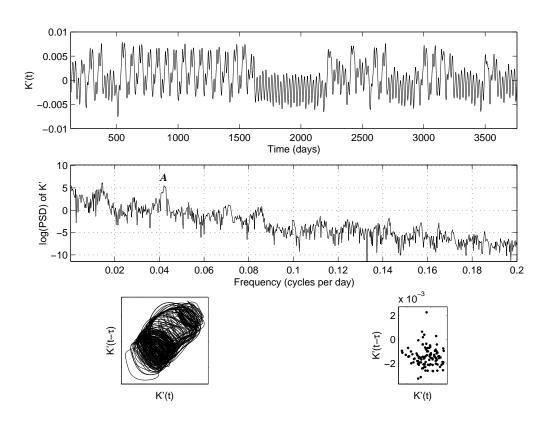
Figure 17: Time dependence of K' with  $Ro = 2.85 \times 10^{-2}$  for an integration started from branch 1 initial conditions. Top: time series; middle: power spectrum of time series (the zero frequency peak has been suppressed); bottom left: delay-space trajectory for the time series; bottom right: Poincaré section of the delay-space trajectory.
