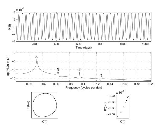
Figure 7: Time dependence of K' with  $Ro = 1.0 \times 10^{-2}$ . Top: time series; middle: power spectrum of time series (the zero frequency peak has been suppressed); bottom left: delay-space trajectory for the time series; bottom right: Poincaré section of the delay-space trajectory.
