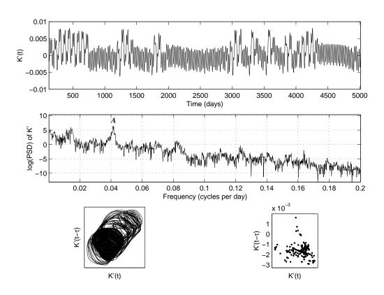
Figure 16: Time dependence of K' with  $Ro = 2.80 \times 10^{-2}$  for an integration started from branch 1 initial conditions. Top: time series; middle: power spectrum of time series (the zero frequency peak has been suppressed); bottom left: delay-space trajectory for the time series; bottom right: Poincaré section of the delay-space trajectory.
