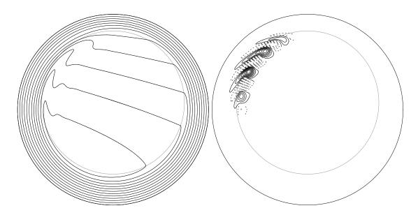
Figure 8: Contours of  $\psi$  averaged over one oscillation (left) and the difference in  $\psi$  from this field at one time (right; the contour interval has been reduced by a factor of 30).  $Ro = 9.5 \times 10^{-3}$ ; contours of negative  $\psi$  are dashed and the grey ellipse marks the bottom of the slope. North is at the top and the mean flow is clockwise.
