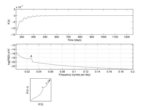
Figure 6: Time dependence of K' with  $Ro = 7.5 \times 10^{-3}$ . Top: time series; middle: power spectrum of time series (the zero frequency peak has been suppressed); bottom left: delay-space trajectory for the time series.
