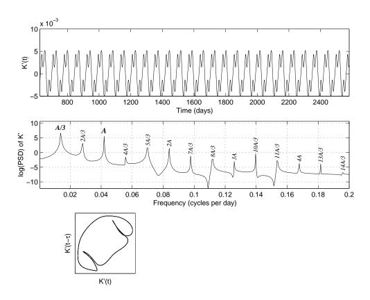
Figure 13: Time dependence of K' with  $Ro = 2.75 \times 10^{-2}$ , on branch 2. Top: time series; middle: power spectrum of time series (the zero frequency peak has been suppressed); bottom left: delay-space trajectory for the time series.
