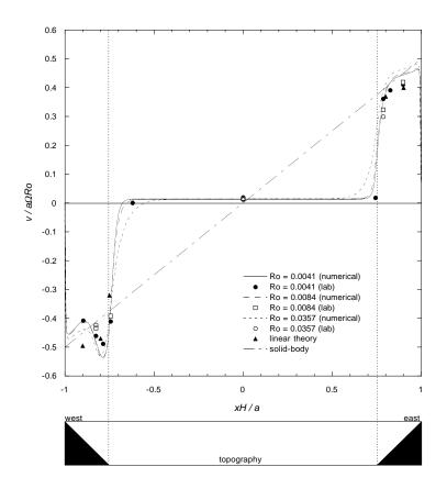
Figure 2: Laboratory and theoretical results from [Griffiths and Veronis, 1997] and [Griffiths and Veronis, 1998] compared with numerical results for the northward component of the normalized velocity as a function of position along the line y = 0, for cyclonic forcing.
