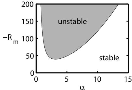
Figure 2: Stability of perturbations with Rayleigh number  $R_m$  and wavenumber  $\alpha$ .
