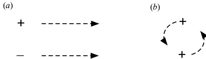
Figure 3: Schematic showing point vortex pairs: (a) two vortices of equal and opposite circulation, translate without changing their separation; (b) two vortices of equal circulation, rotate without changing their separation.
