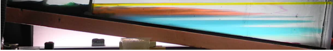
Figure 5: Fingering intrusion observed for N = 1.9 , \rho_0 = 1.2 , \theta = 8.4 , d = 13 - 45 \mu\text{m} and h_0 = 6 \text{ cm} (blue dye). Note: the red and yellow dye are previous lock exchange experiments run in the same tank set-up, but have not affected the overall stratification of the ambient and so do not affect the results presented here.
