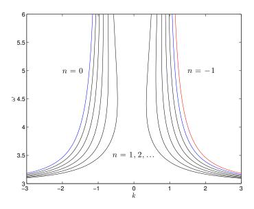
Figure 5: Dispersion curve for evanescent waves  $(|\omega| > N)$ . The red line is the Kelvin mode, the blue lines are the n = 0 modes, and the black lines are the n = 1, 2, ... modes.
