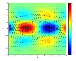
(c) A westwards propagating inertio-gravity wave with large positive  $\omega$ , k = -1.
