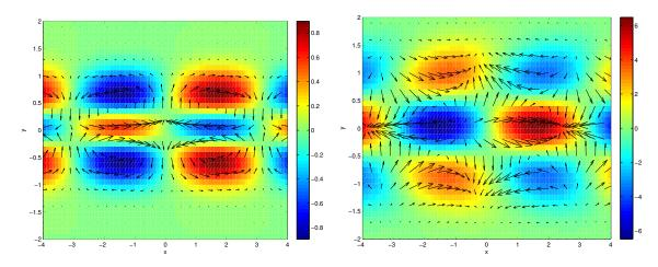
(a) A westwards propagating Rossby wave with (b) An eastwards propagating inertio-gravity wave small positive  $\omega$ , k = -1. with large positive  $\omega$ , k = 1.
